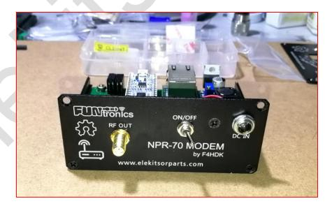
Take out the front panel and secure it to the bottom cover, then following the instructions we just made for L4940, secure the LM2937's heat sink plate to the front panel.
