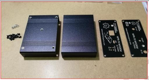
Find out supplied enclosure from the package, insert the modem board to the bottom cover of the enclosure by the slot on the wall. Locate the rear panel, mount the DC port and toggle switch onto the panel, and finally the rear panel onto the bottom cover. Please note that you may need to adjust the nut on the SMA port backward in order to fit our modem board rightly inside the enclosure. See the pictures below for the details.
