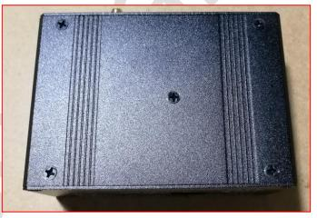
Now it is almost done, locate the top cover, put the top cover on and secure it with 4 screws. Pay attention when installing the top cover, there are groove or bump on the 2 vertical walls, and the bottom cover as well. The bump on the top should touch the groove on the bottom cover, vice verse.
